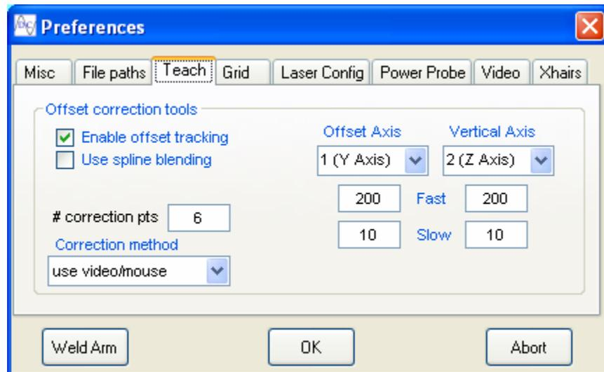
**Enable offset tracking** enables/disables the tracking feature.
