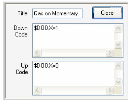
There is an **On code** and an **Off code** either of which can be programmed or left blank. If you wish to have a button that only turns a gas valve on while you hold it down, you would set the On code to \$D00.X=1, then the Off code to \$D00.X=0.
