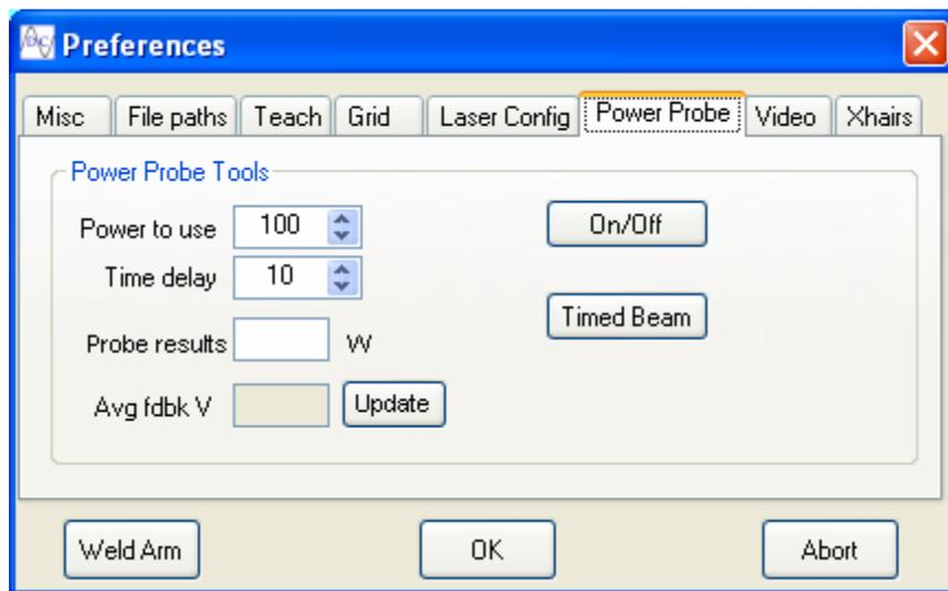
Press the check mark button for some calculations, and if you wish to use the newly calculated Feedback Watts/Volt value, simply press Ok.
