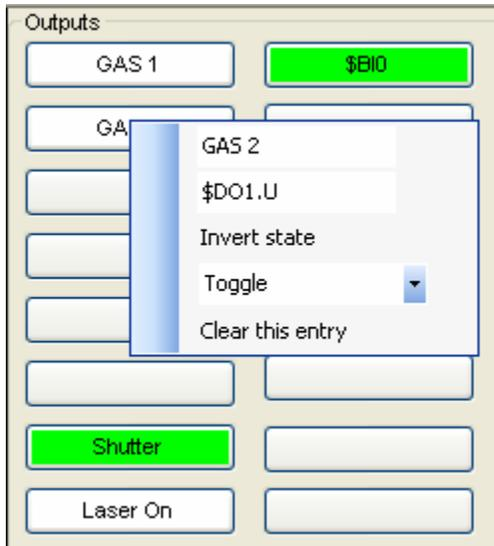
The first line is the button's title, here it's GAS 2. On the second line is the IO address. Here it's a digital output on the U axis. It can be any valid \$DO or \$BO point.
