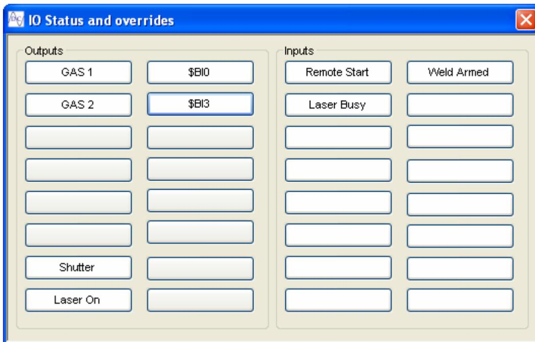
The Remote Start input is required if you wish to use a footswitch or other remote switch tied to one of the system's inputs. It can be either a \$DI or \$BI definition, it just has to be named Remote Start. See Run Tab for more information on the Remote Start input.
