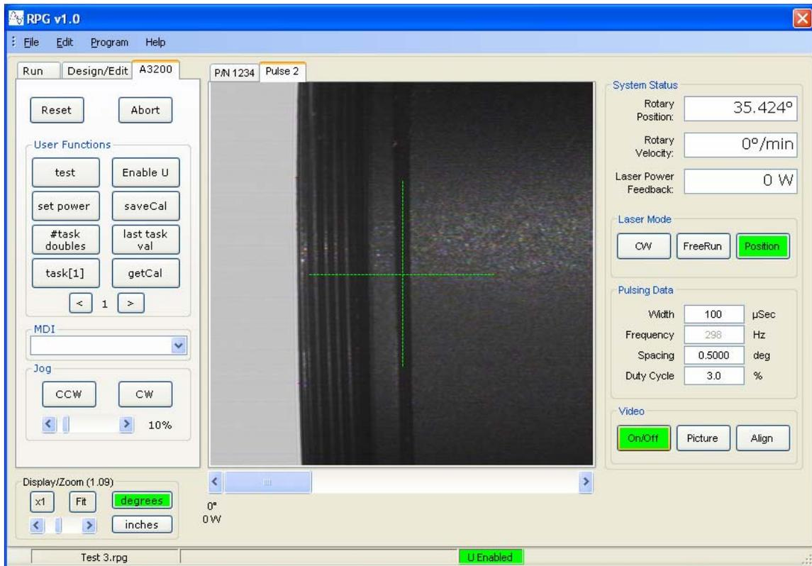
With the Video Tools option installed, your display can also be used as a live video display from your system (or off axis camera). Use the Video group of buttons to control the video display. See Preferences, Video tab for setup information.
