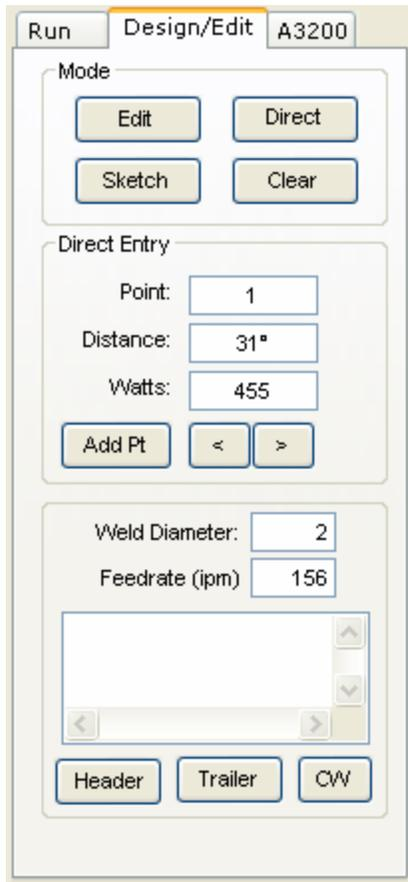
*NOTE: You can use + and – before a value entered in either the distance or watts box to specify an incremental distance from where that point currently is. ( +10 moves 10 degrees right)*
