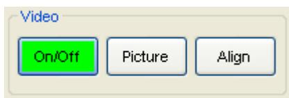
Video display is on and live video is active. Toggle this on/off to switch between program view and live video.
