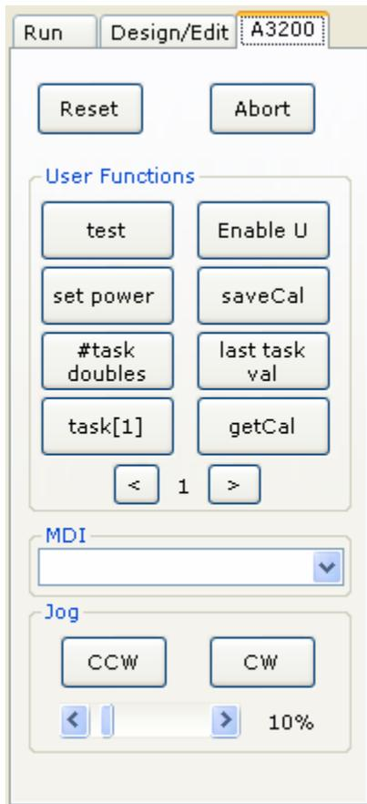
**Reset** button causes a hard reset of the A3200 system. This may take a few seconds.
